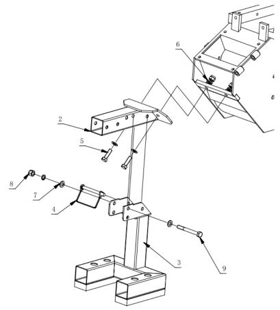
5. Assemble the tow bar on the foot frame(spring washer, flat washer\*2, M10\*70, lock nut)\*2
