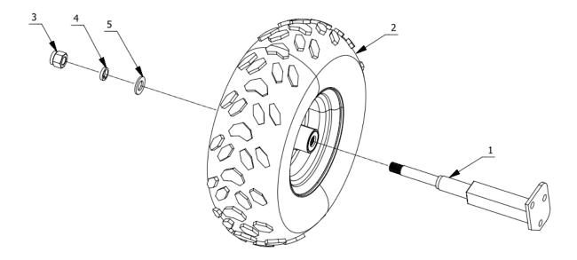
b. Locate the 2 wheels and the correct hardware needed to assemble the wheels (M10\*30 bolt, spring washer, flat washer\*2, lock nut)\*6
