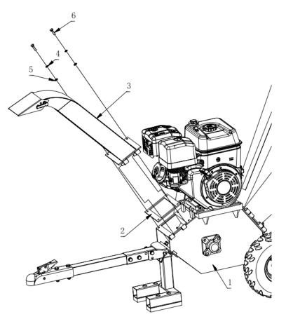
7. Connect the emergency stop wire located at the base of the hopper coming from the engine. This can be done by inserting the bullet male wire into the bullet female wire connector.
