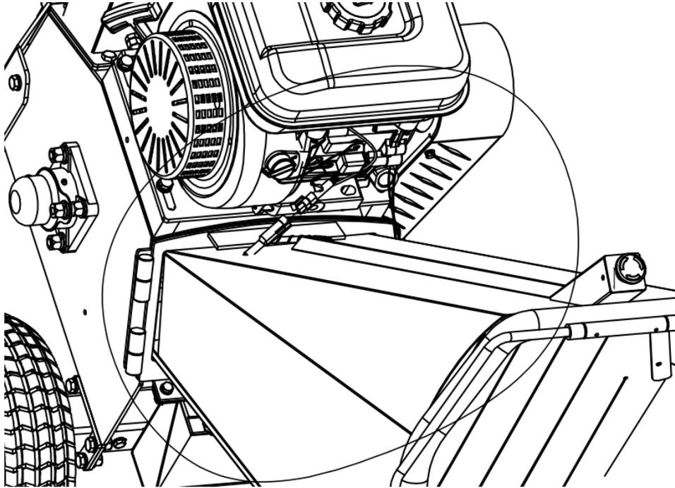
8. Assemble the battery and its wires (optional, electric start only) (M8\*25, flat washer\*2, spring washer, lock nut)\*2, (M6\*15, M6 nut)\*2
