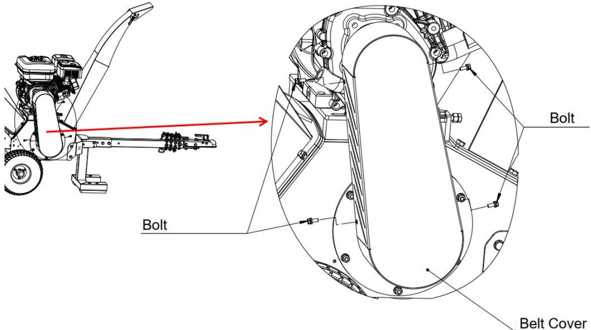
**Step 2: Remove the old belts and replace with new belts.**
