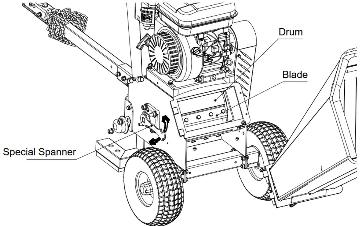
Step 3: **(WITH CAUTION)** Use the "T-Socket" tool to unscrew the 5 "Blade bolts". Once the blade is replaced and in position, tighten the 5 "Blade bolts".
