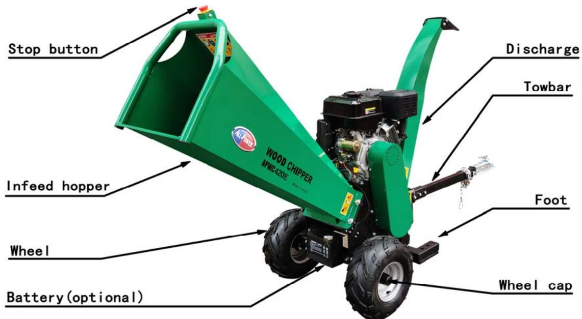
1. Unpack the machine from the crate, the parts you find will be as the below figure shows:
