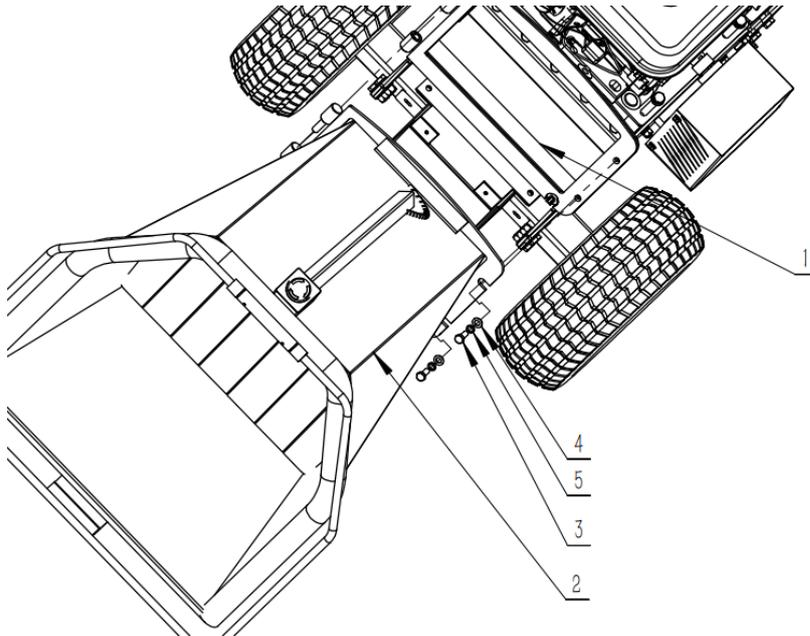
4. Assemble the foot frame and install onto the wood chipper base (M10\*25 bolt, flat washer\*2, spring washer, lock nut)\*4, (M10\*80 bolt, flat washer, spring washer, lock nut, pin)
