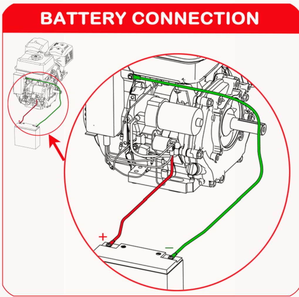
**\*If your chipper is electric start model, connect the battery as the figure shows.**
