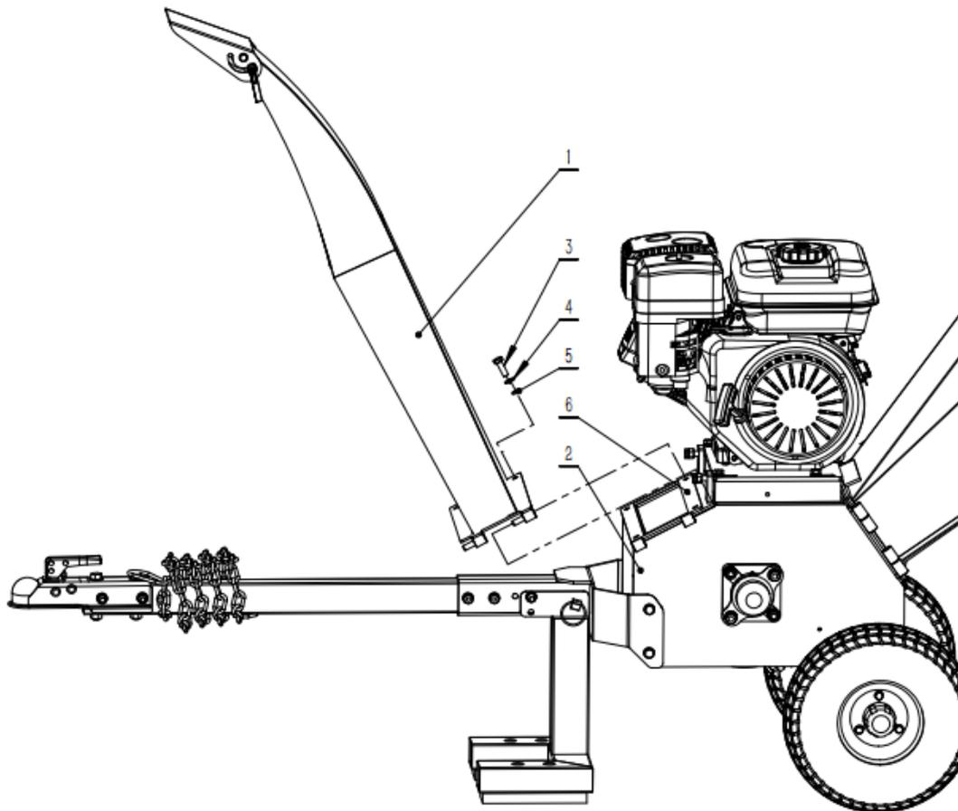
7. Connect the emergency stop wire located at the base of the hopper coming from the engine. This can be done by inserting the bullet male wire into the bullet female wire connector.
