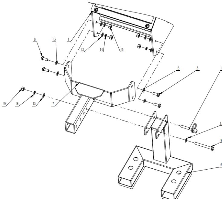
5. Assemble the tow bar on the foot frame(spring washer, flat washer\*2, M10\*65, lock nut)\*2
