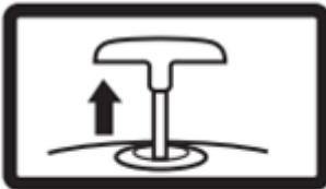
6. When starting engine, pull cord slowly until resistance is felt then pull rapidly to avoid kickback.
