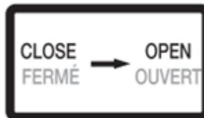
7. Open the choke after pressure washer has started.
