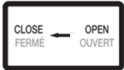
5. When cold-starting, close the choke. When warm-starting, open the choke.
