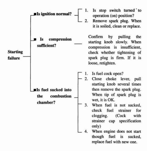
When the engine does not start in spite of above mentioned inspection, ask the distributor or repair factory for inspection.
