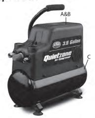
The pressure switch (located internally) shuts down the motor and relieves air pressure in the pump and transfer tube when the air pressure in the tank reaches the kick-out pressure. As compressed air is used and the pressure level in the tank drops to the kick-in pressure, the pressure switch restarts the motor automatically, without warning, and the pump resumes compressing air.
