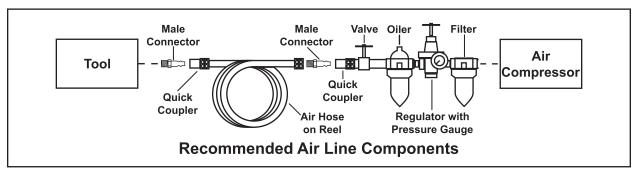
**TO EXTEND THE LIFE OF YOUR AIR TOOLS AND EQUIPMENT,** it is recommended to install an oiler and water filter in series with the Air Output Line of the Air Compressor.
