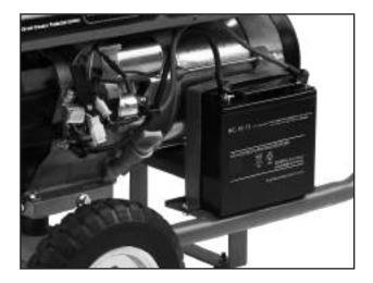
Put the battery on the frame, have the battery assembled with the provided accessories as shown.
